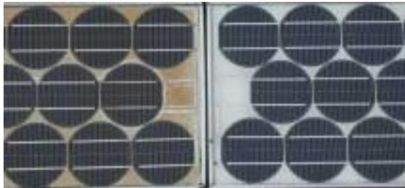
**Figure 8:** 21-year old module ASI16-2300 (ARCO Solar Inc.).
